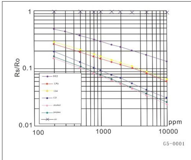
Ordinate means resistance ratio of the sensor ( $R_s/R_o$ ), abscissa is concentration of gases.  $R_s$  means resistance in different gases,  $R_o$  means resistance of sensor in 1000ppm Hydrogen. All test are under standard test conditions.
