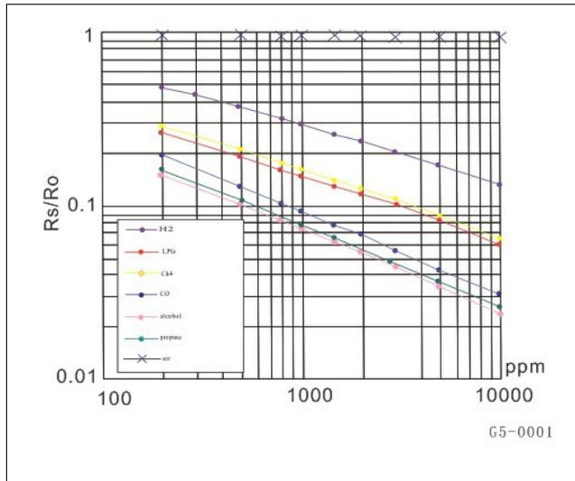
Ordinate means resistance ratio of the sensor ( $R_s/R_o$ ), abscissa is concentration of gases.  $R_s$  means resistance in different gases,  $R_o$  means resistance of sensor in 1000ppm Hydrogen. All test are under standard test conditions.
