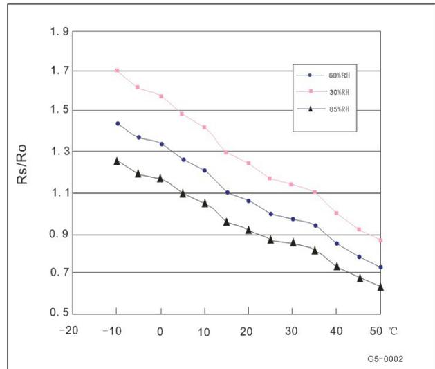
Ordinate means resistance ratio of the sensor ( $R_s/R_o$ ),  $R_s$  means resistance of sensor in 1000ppm Butane under different tem. and humidity.  $R_o$  means resistance of the sensor in environment of 1000ppm Methane, 20 °C /65%  $R_H$
