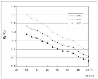
Ordinate means resistance ratio of the sensor (Rs/Ro), Rs means resistance of sensor in 1000ppm Propane under different tem. and humidity. Ro means resistance of the sensor in environment of 1000ppm Propane, 20 °C /&5 % R  $_{\rm H}$
