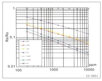
Ordinate means resistance ratio of the sensor (Rs/Ro), abscissa is concentration of gases. Rs means resistance in different gases, Ro means resistance of sensor in 1000ppm H2.All test are under standard test conditions.
