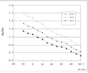
Ordinate means resistance ratio of the sensor (Rs/Ro), Rs means resistance of sensor in 1000ppm Methane under different tem. and humidity. Ro means resistance of the sensor in environment of 1000ppm Methane,  $20^{\circ}C/65\%$  R<sub>H</sub>
