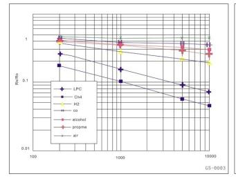
Ordinate means resistance ratio of the sensor (Rs/Ro), abscissa is concentration of gases. Rs means resistance in different gases, Ro means resistance of sensor in 1000ppm Methane.All test are under standard test conditions.
