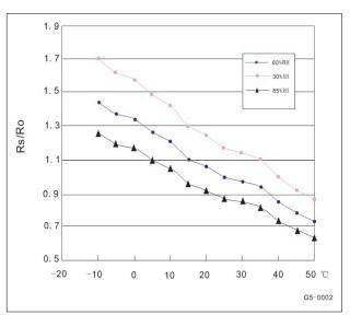
Ordinate means resistance ratio of the sensor (Rs/Ro), Rs means resistance of sensor in 000ppm Butane under different tem. and humidity.Ro eans resistance of the sensor in environment of 1000ppm Methane,  $20^{\circ}C/65\%R_{H}$
